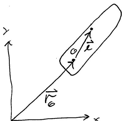
$$\text{Fart } \vec{V} = \left[ \frac{dx}{dt}, \frac{dy}{dt} \right] = [V_{0x} - l \cdot \omega \sin \theta, V_{0y} + l \cdot \omega \cos \theta].$$
