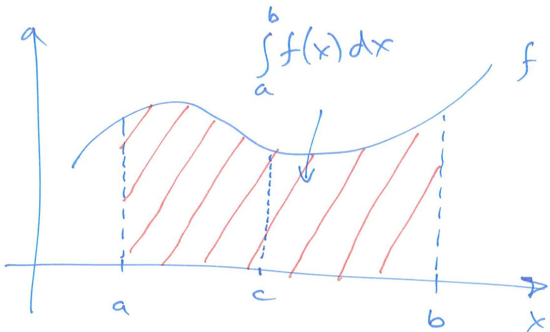
$$\int_a^b f(x) dx = \int_a^c f(x) dx + \int_c^b f(x) dx$$
